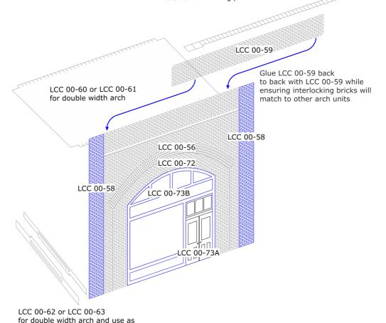
TO ASSEMBLE ARCH UNIT IN LOW RELIEF
